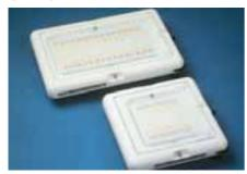
Horizontal developing chambers permit the number of samples to be doubled when compared to a vertical tank. Plates are developed from opposite sides simultaneously towards the middle.
