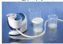
The Sentino™ pump system is ideal for microbiological MF technique using Pall MicroFunnel™ filtration units. Designed to use peristaltic action to draw the sample through the filter and send filtrate directly to drain or waste collection. The housing is a PC ABS-blended polymer, the keypad and label PE, the pump head PEI with PTFE-filled PBT rollers. The fluid path adaptor is PP.
