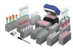
Grant blocks have a depth of 63 mm, ensuring precise temperature control for test tube applications.
