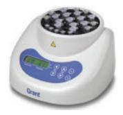
Compact digital block heater with fixed circular block. Unit features digital control, two line display allowing simple and accurate setting of temperature and time, plus display of current status while in operation. The aluminium block is housed in durable and easy to clean, chemically resistant plastic. Unit has a 0.1 °C display resolution.
