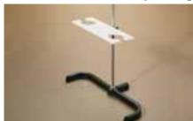
PU coated cast iron stand 200×450 mm, steel rod 500×12 mm, bosshead and holder for two funnels.
