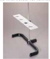
$PU\ coated\ cast\ iron\ stand\ (200\times450\ mm),\ steel\ rod\ (500\times12\ mm),\ bosshead\ and\ holder\ for\ four\ funnels.$
