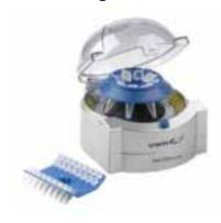
This centrifuge was developed for applications that do not require high speed centrifugation, such as microfiltration and cell separation, and can also be used in a cold room. Metal base with ABS body and transparent safety cover. On closing the lid, the rotor quickly accelerates to maximum speed. Pressing the button on the front of the unit stops operation and opens the lid. Alternatively, the unit can be turned on and off with the switch at the back.
