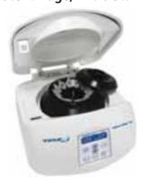
Safe and easy to use centrifuge delivering optimum performance in a compact unit. All operating parameters, including rpm, RCF and remaining time, are set and displayed digitally. It has an automatic lid release, pulse spin function for fast, convenient quick spins and an unique internal airflow design to reduce the heating up of samples.
