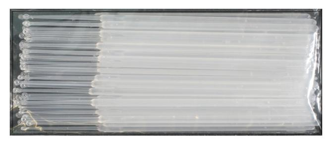
Manufactured from polypropylene these loops are available in both 1µl and 10µl t0 suit your requirements. A needle version is also available.
