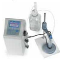
These automatic potentiometric titration analysers are specifically designed to determine pH and total acidity in a variety of food and beverage applications, providing a compact and reliable solution for routine QC analysis measurements.
