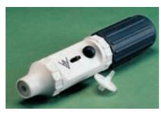
Allows comfortable control of the filling, volume adjustment and dispensing of liquids through thumb-operated controls. For one mark and graduated pipettes from 0.1 to 100 ml (accommodated by silicone adapter). With fine level adjustment and blow through for blow-out pipettes.
