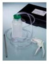
Hand operated vacuum pump sampler, equipped with a 2,5 metre long PVC hose, the stainless steel weight will sink the end of the hose to the required sampling depth. Liquid only comes into contact with the suction hose and sample bottle.
