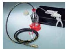
Glass bottle and hose are connected in such a way that they conduct electricity and are grounded via a grounding cable. Operation: Ground the device, immerse the suction hose to the required depth, attach the adapter to the sampling bottle, generate a vacuum with the manual pump and collect the sample, remove the filled sampling bottle, close it and label it.
