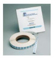
Self-adhesive, non-toxic, chemical process indicators change from blue to pink upon exposure to 10 minutes of saturated steam at 121  $^{\circ}$ C or 2 minutes at 134  $^{\circ}$ C. Longer exposure will result in a brighter shade of pink. The blue to pink colour transition is sensitive to time, temperature, and the presence of saturated steam.
