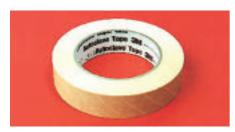
The colour of the sensitive ink changes after sterilisation. The adhesive tape indicates that the expected temperature was reached during the sterilisation process.
