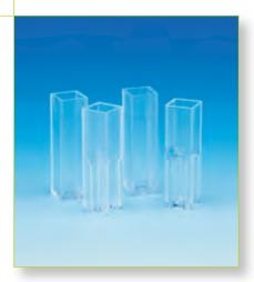
Sterilin Cuvettes are suitable for use with most spectrophotometers for water analysis or chemistry and life science applications.
