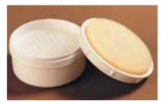
The mercury globules are absorbed by the foam pad. A mesh inside squeezes the mercury out of the foam, so it is immediately ready for use again.
