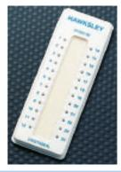
For sealing capillary tubes. The dry end of the filled tube is pressed into the Cristaseal with a twisting motion producing a firm seal with flat boundaries. The tray may be used as a carrier for tubes prior to centrifuging.
