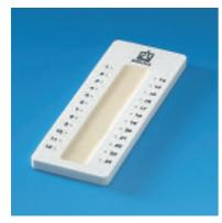
Non-drying vinyl putty on a plastic tray. For rapid sealing of several hundred micro haematocrit capillaries. Up to 24 capillaries can be placed vertically in numbered positions along the sides of the tray.
