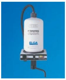
This wall mounted disposable deioniser produces water up to a quality of 10M.-cm at flows of up to 90 l/hr. Designed for users with a requirement for low volumes deionised water, the Micromeg requires no electrical input as its water quality meter is battery operated.
