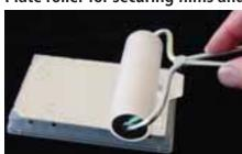
Soft rubber roller recommended for assuring tight and consistent application of adhesive films to microplates.
