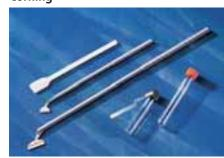
Useful for the manual harvesting of cells, scrapers are designed for use in flasks and cell lifters for use in harvesting cells (especially stem cells) in dishes.
