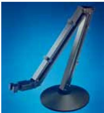
Electrode arm moves smoothly in almost any direction, holding up to 4 electrodes + 1 temperature sensor safely and securely in selected positions. Fingertip control raises, lowers, and pivots the holder. The arm articulates at three points while maintaining electrodes in a vertical position.
