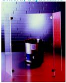
Acrylic shield with 1 front plate (H/W) 700/500 mm and 2 side plates (H/W) 700/180 mm, 10mm thick. Providing protection against fragments and splashes. The side plates can be twisted up to an angle of 120°.
