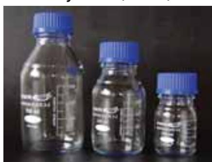
Grade 3.3 borosilicate glass with PP screw cap
