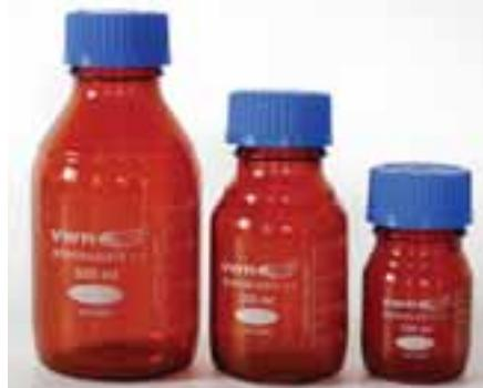
Amber borosilicate glass with PP screw cap
