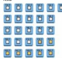
These thermometer strips are made of self-adhesive foils with temperature sensitive elements for temperature control and regulation. They are used for measurements on moving and/or small parts and for long-term monitoring.
