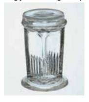
Soda-lime glass. With grooves, to accept ten 76×26 mm slides, vertically, back to back.
