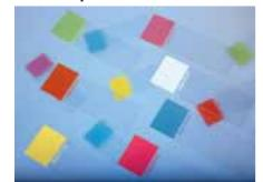
These microscope slides come with a light opaque coating in different colours. Each colour codes different specimens at a glance according to urgency, processing or staining technique, etc.
