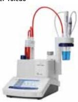
This reliable titrator is designed for basic routine applications and titrations in the analysis of food, water and chemicals. The One Click™ user interface is optimised for direct access to all routine tasks and provides clear information to the user. It offers four shortcut buttons for immediate start of routine operations and user-specific home screens with customisable shortcuts and user-defined operation languages.
