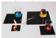
These plates made from ceramic glass protect high quality surfaces from high temperature containers, such as crucibles, evaporating dishes, glass containers and more. They also provide reliable protection against deep frozen items. Feet at the edges of the plates prevent direct contact with the surfaces to be protected.
