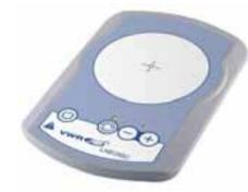
Extremely flat and compact magnetic stirrer with no moving parts. Reverses direction of rotation every 30 seconds to ensure optimum mixing.
