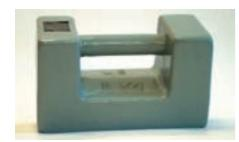
Rectangular weights made from cast iron (density 7.2 g/cm<sup>3</sup>).
