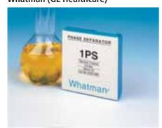
High grade filter paper impregnated with a stabilised silicone that renders it hydrophobic, retaining the aqueous phase and passing the solvent phase through.
